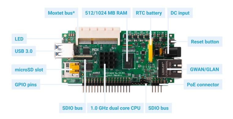
MOX A is available in two variants – 512 MB RAM and 1024 MB RAM. The first one is included in the MOX Pocket Wi-Fi, Power Wi-Fi and Classic, the second one in the MOX Start, which is the starting point for a customized network solution composed of Turris MOX components.
